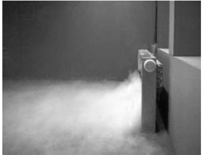
Air flow pattern: Cooling operation
