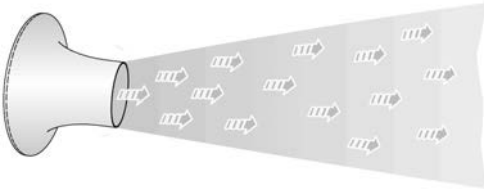
Fig. 23: Horizontal air discharge, isothermal
