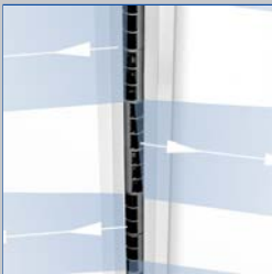
Alternating horizontal air discharge
