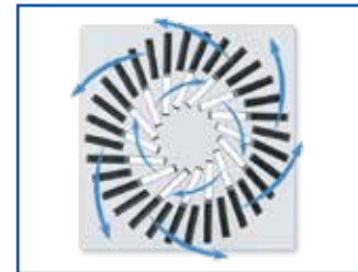
Outer air control blades set to external swirl, inner blades set to internal swirl
